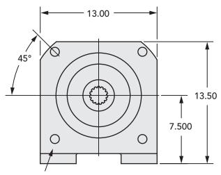
(4) 1.0-8 UNC  $\times$  2.0 Deep Equally Spaced on a 13.781 Diameter Bolt Circle Input End Only
